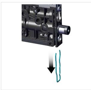
3. Then remove the silencer and silencer insert from the ejector.
