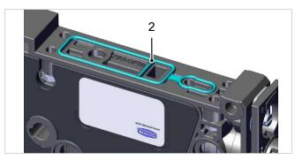
6. Check that all nuts (4 pieces) are fitted ①. Attach the housing plate (1) to the ejector housing in the correct position and tighten the four fastening screws with a tightening torque of 0.25 Nm ②.
