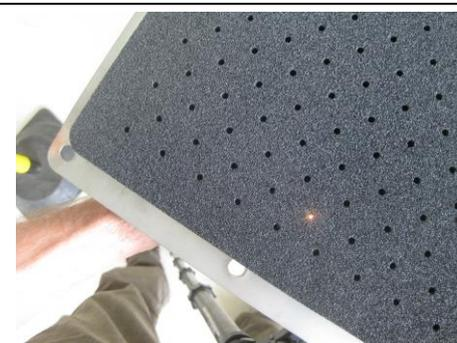
**(10)** Check flush of the holes by using light
