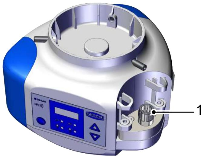
The ECBPi is electrically connected to the higher-level machine or controller (the voltage supply and the transfer of the input and output signals) using the enclosed connection cable with an 8-pin M12 connector via the interface (item 1).
