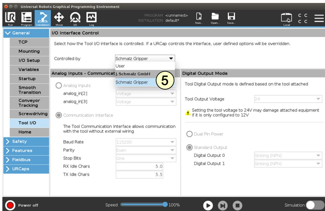
**(5) UR CB series:** Select the “Schmalz Gripper” device configuration from the drop-down menu under “Installation > I/O”.
