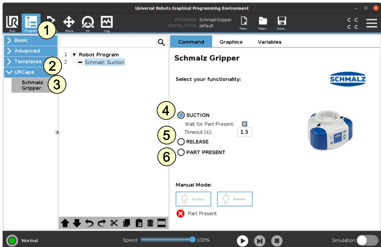
(5) "RELEASE": Workpiece is released (deactivate suction)
