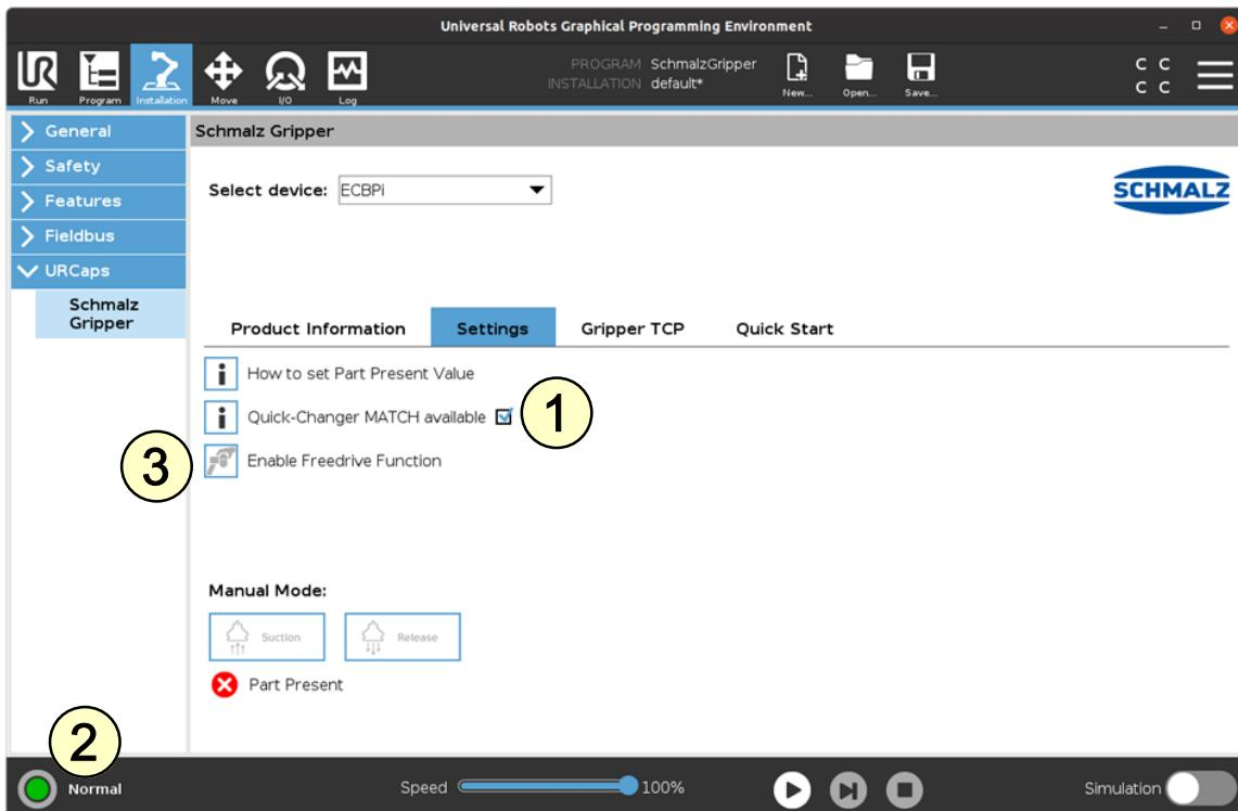
1. Activate the button to enable the Freedrive function (3) under "... > Settings".
