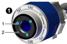
1. Loosen the screws (1) (x 3) with a size 2.5 Allen key **1** and remove the profile disk (2) **2**. Retain the profile disk (2) and the screws (1) to re-use.
