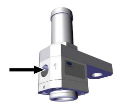
Connect the compressed air for the "suction" function to the G1/8" thread labeled with the number 1. The compressed air connection (inlet) for supplying the blow-off function is labeled with the number 12, as shown in the figure.
