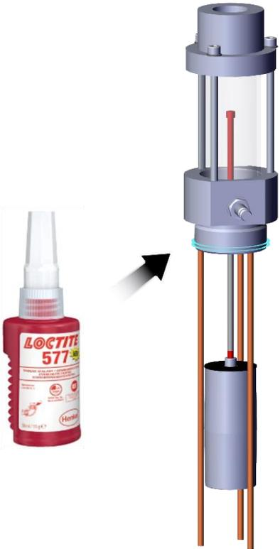
Step 11: Insert new float using an open-ended wrench (size 50) or a pipe wrench
