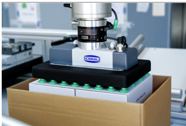
Area gripping system FQE-V Xc when palletizing cardboard boxes
