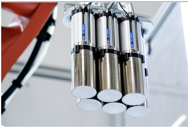
Magnetic gripper when handling round battery cells
