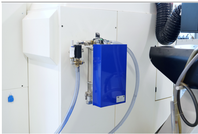
Liquid separator NLS in use on a CNC machining center
