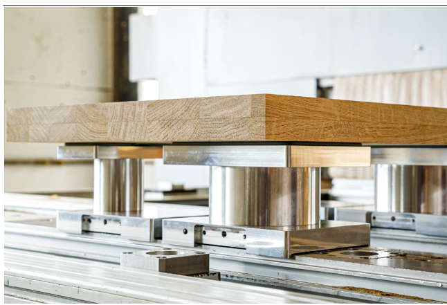
Vacuum block VCBL-K2-HD when clamping solid wood
