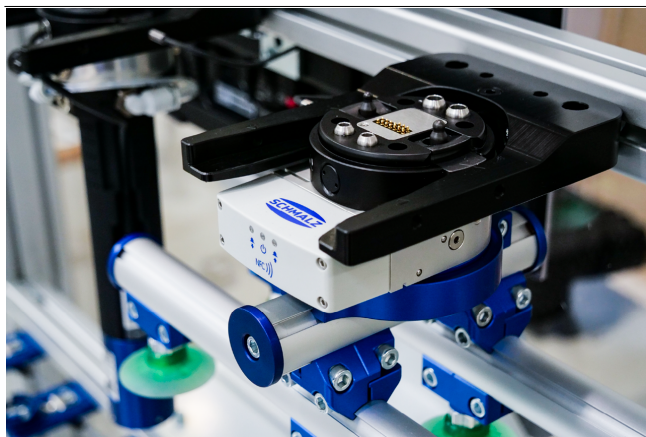
Pneumatic vacuum generator RECBi MATCH when handling carton packages
