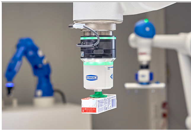
Electrical vacuum generator ECBPMi MATCH when handling small cartons
