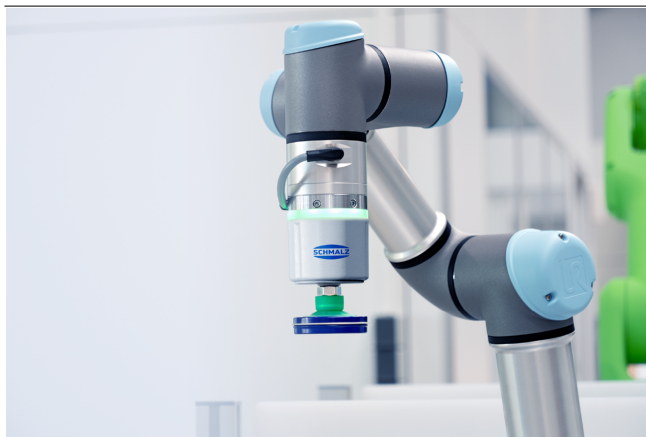
Electric vacuum generator ECBPMi for handling cans
