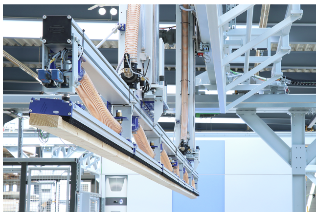
Area gripping systems FMP-S for layer-wise stacking of construction wood
