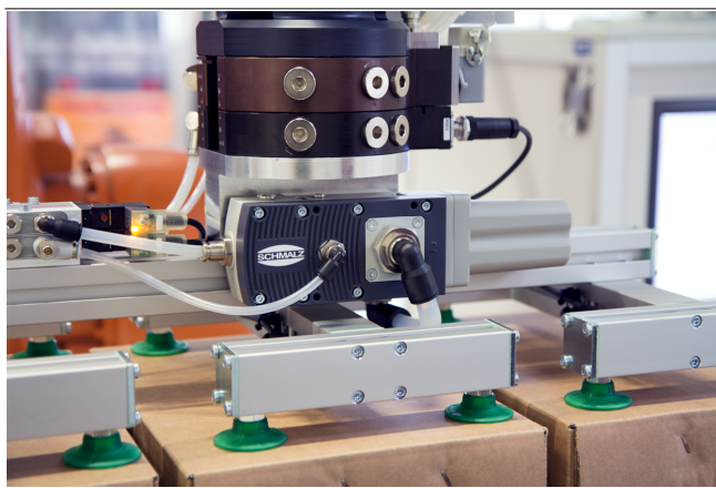
Central vacuum generation with basic ejectors SBPL
