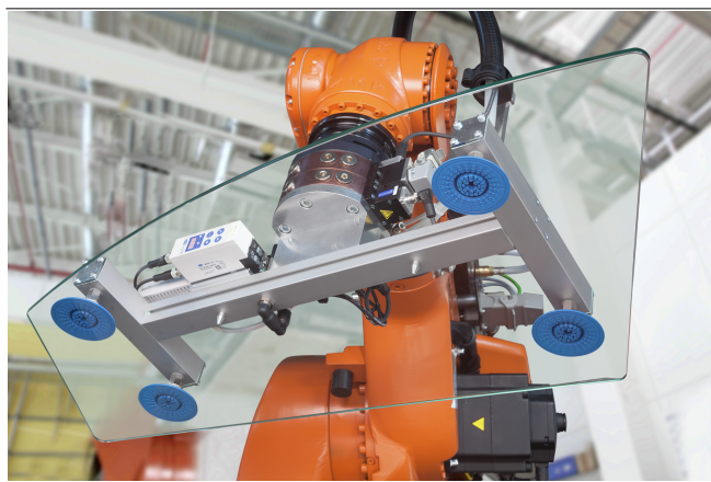
Central vacuum generation by compact ejectors X-Pump SXPi / SXMPi
