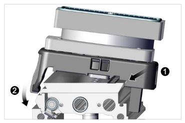
The vacuum block is not fixed in place. It can be positioned on the console by moving it. The vacuum block is only fixed to the console when the console's compressed air circuit is activated.
