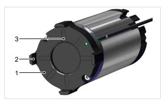
In the case of the standard gripping element with four guide pins, it is no longer possible to ensure that the device can pick up and set down accurately when the wear limit is exceeded. The degree of wear can be determined through the six slots (3) on the underside.
