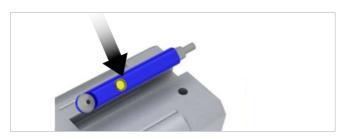
2. Push the sensor to the stop of the T-slot, or in the case of variants with **open T-slot**, fix the sensor flush with the lower end of the slot (towards the gripping surface).
