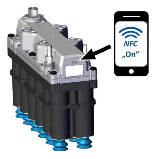
The reading distance is very short for NFC applications. Determine the position of the NFC antenna in the reading device used. If parameters of the device are modified via IO-Link or NFC, then the power supply must subsequently remain stable for at least three seconds to prevent data loss.
