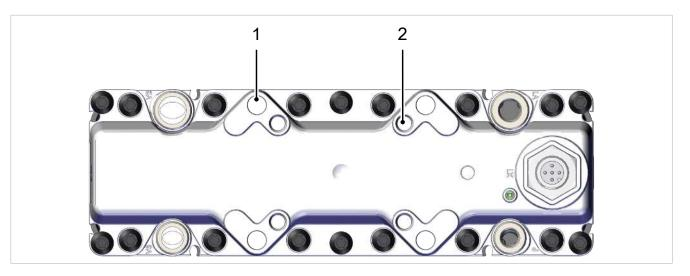
The four holes at position (2) are used to mount positioning pins with a diameter of 5 mm. The use of positioning pins increases the accuracy of the position of the FMG on the handling system (especially when replacing individual modules).
