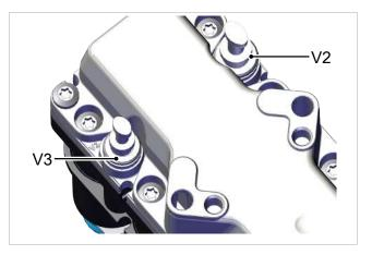
To ensure the safe operation of the gripper, the vacuum generator used should provide a suction capacity of approximately **36 liters per minute**.
