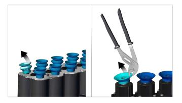
• Remove the damaged suction cup from the nipple by hand or with a gripper.
