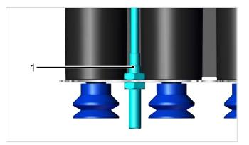
1. Install the sensor on the mounting hole (1) with a 5.8 mm diameter.
