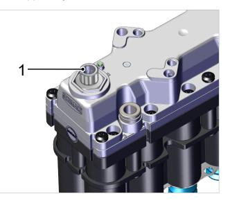
Attach the connection cable to plug position
