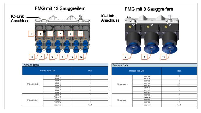
The input data (Prozess Data In) is not used with this device.
