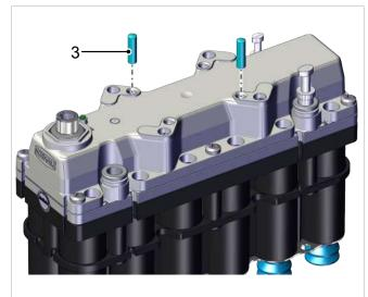
1. Insert at least two positioning pins (3) into the bores (2).
