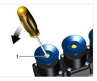
1. Use a sharp tool to pierce the sieves (1) and pry them out of the holes.
