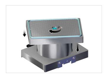
▶ Then tighten the screw again with the specified torque of 30 Nm.
