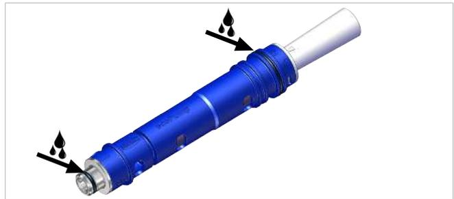
2. Ensure that the ejector module (4) is in the correct position and push it into the opening until it stops, with the suction openings of the ejector module (4) as shown.
