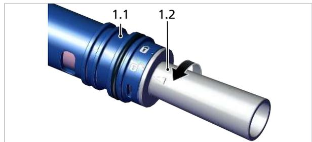
2. Pull the nozzle fitting (1.2) out of the main body (1.1), pulling only in the axial direction.
