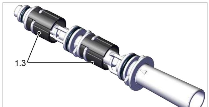
5. Grease the O-rings slightly before mounting the ejector module.
