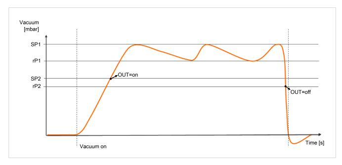
The diagram below shows the vacuum curve when the control function is activated:
