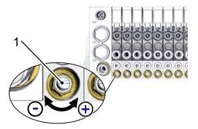
The blow-off flow rate is set to 100% (opened 2 turns) when delivered.
