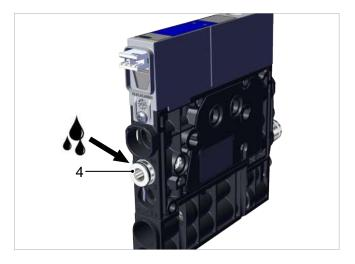
7. Before mounting the ejector/valve or dummy plate, check the position and condition of the O-rings.
