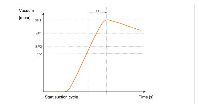
The measured evacuation time t1 can be read out using the "Evacuation time t1 for ejectors" parameter 0x0095.
