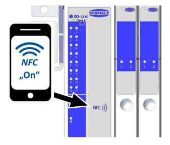
The reading distance is very short for NFC applications. Determine the position of the NFC antenna in the reading device used. If parameters of the device are modified via IO-Link or NFC, then the power supply must subsequently remain stable for at least three seconds to prevent data loss.
