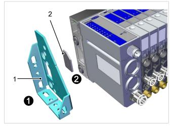
2. Remove the mounting bracket (1) ① and remove the silencer (2) ②.
