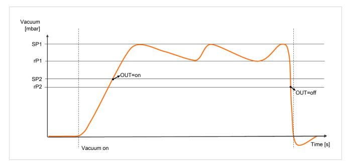
The ejector has an integrated air saving function and automatically regulates the vacuum in suction mode:
