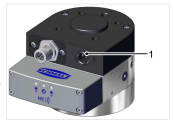
Connect the compressed air hose for supplying the integrated vacuum generation via the compressed air connection (1) (marked with 1). Use a maximum tightening torque of 2.5 Nm.
