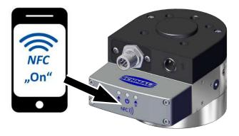
The reading distance is very short for NFC applications. Determine the position of the NFC antenna in the reading device used. If parameters of the device are modified via NFC, then the power supply must subsequently remain stable for at least three seconds to prevent data loss (error E01).
