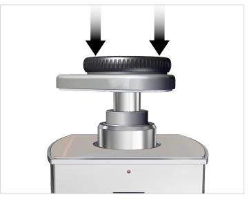
2. Releasing the catch of the quick adjustment mechanism: Clasp the clamping disc with both hands and press and hold the locking disc down by about
