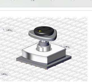
4. Place the mechanical clamp on the grid table. Make sure that there is an open vacuum feedthrough in the grid table within the sealing frame.
