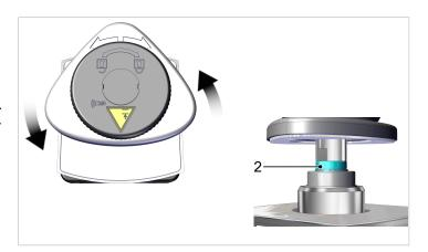
The clamping disc with the screwed-on extension (1) is released.
