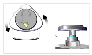
⇒ The clamping disc with the screwed-on extension (1) is released.
