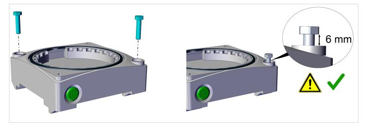
✓ At least two M6x16 screws are mounted diagonally in the mount with a clearance of 6 mm.
