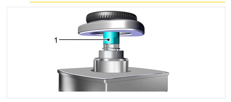
The VCMC QUICK is delivered as standard with the extension (1) mounted.
