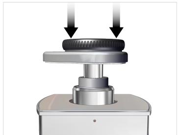
⇒ This releases the quick-locking mechanism.
