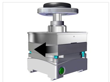
3. Tighten at least two M6 hex head screws (SW10) with a tightening torque of 5 Nm.
