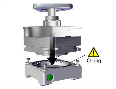
2. Turn the suction cup clockwise until the bayonet recess abuts on a screw.
