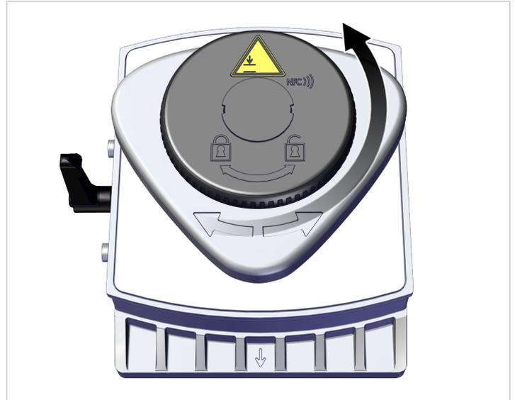
2. **Releasing the catch of the quick adjustment mechanism:** Clasp the clamping disc with both hands and press and hold the locking disc down by about 4 mm.
