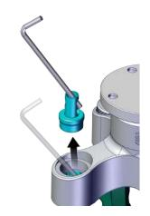
3. Remove the gripping finger from the holder in the direction shown.
