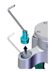
3. Remove the gripping finger from the holder in the direction shown.
