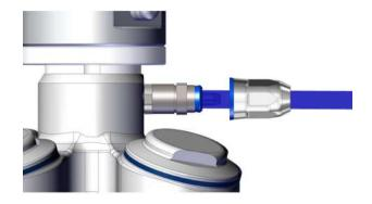
6. Push the sealing ring (4) up to the clamping element (3).
