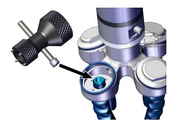
3. Unscrew the lock washer using the four pins on the multitool (turn counterclockwise).
