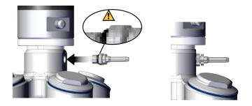
3. Push the union nut (5), the sealing ring (4) and the clamping element (3) (in this order) on to the hose.
