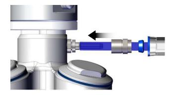
5. Screw the clamping element (3) on to the inner pin (2) as far as it will go. Tool: Hexagon wrench SW13.
