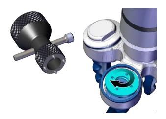
3. Press the clamping element with the thread on the multitool in the correct position (internal thread pointing upward) into the opening provided in the gripping finger until it is seated in the groove on the lock washer.
