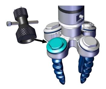
2. Remove/pull out the clamping element using the thread on the multitool.
