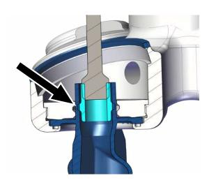
4. Screw in the cover cap using the multitool, tightening torque 8 Nm.
