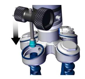
⇒ The clamping element sits in the groove in the lock washer.
