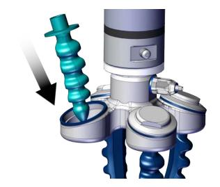
2. Fit the lock washer using the multitool, tightening torque 7 Nm.
