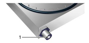
Connect the vacuum hose with an outside diameter of 6 mm to the hose connection (1) with a plugin screw union.
