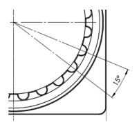
Place the vacuum blocks on the Adapter-Plate. The vacuum block VCBL-B that is used can be placed into the suction cup mount of the Adapter-Plate in 15° steps to align the suction area as desired.
