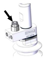
Connect the compressed air connection (inlet) for the integrated vacuum generation supply for the "suction" function using the size-6/4 plug-in screw union.
