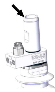
• Connect a hose with a 20 mm inner Ø to the exhaust air outlet.
