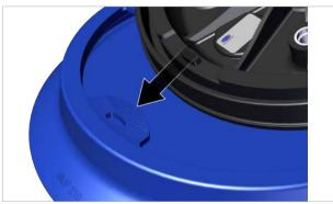
3. Simultaneously fit the sealing ring into the slot and recess on the suction cup connection disc.
