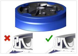
5. Check the tightness of the seal between the sealing ring and the suction cup connection disc.
