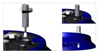
⇒ The touch valve must be screwed in so that the button protrudes at least 1 mm over edge of the sealing ring. This ensures that the button is actuated just before the sealing edge is placed on the workpiece.
