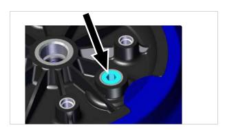
2. For sealing, prepare the male thread in the area displayed on the touch valve with a PTFE strip or low-strength thread lock before mounting.
