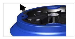
2. Gradually release the sealing ring from the slot using the remaining tabs and detach the suction plate from the suction cup connection disc.
