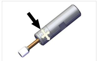
3. Screw the touch valve into the G2 thread until it stops (SW11 hexagonal mid section).
