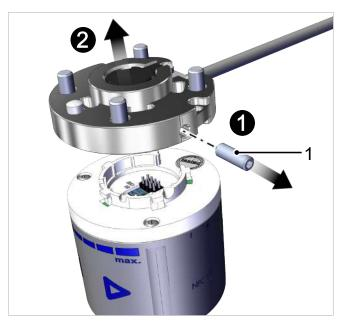
2. Position the flange adapter plate included in the delivery on the suitable collaborative robot using the positioning pin and fasten it using the four M6x12 cylinder head screws. Observe the permitted tightening torque for the thread.
