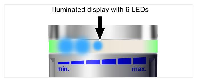
The indicator for the vacuum level that is currently set is activated using one of the buttons.
