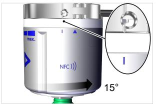
NOTE! End position is not reached and the line on the ECBPMi does not match the groove on the flange. Screwing in the set screw will damage the fiber optics.
