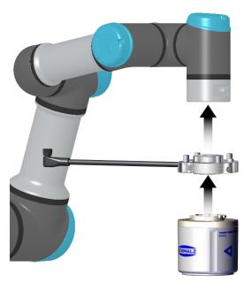
1. Unscrew and remove the set screw (1) 1 to detach the flange adapter plate from the ECBPMi 2.
