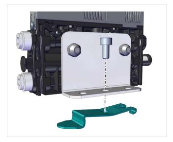
3. Attach the assembly with the bracket onto the DIN rail **1** and press it onto it **2**.
