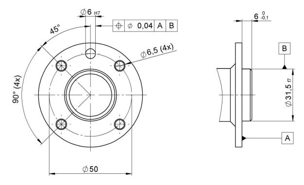
The gripper initially comes equipped with an Ø31.5 f7 base in the corresponding robot flange adapter in order to mount the gripper onto the robot/system.
