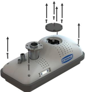
3. Take the two halves of the housing and carefully put them down to the side. Ensure that no hoses or cables on the housing become loose.
