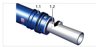
2. Pull the nozzle fitting (1.2) out of the main body (1.1), pulling only in the axial direction.
