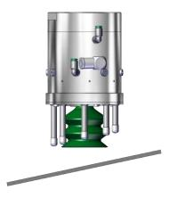
When the workpiece is set up, it must be dimensionally stable or so well supported that it does not become deformed during setup. If the workpiece becomes deformed during setup, the positioning pins will be incorrectly positioned!
