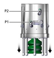
2. Transfer the contour from the workpiece to the positioning pins. I.e. the positioning pins are pushed in to the required position (e.g. by moving the SSCB against the workpiece or by moving the workpiece against the SSCB).
