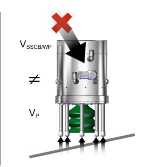
During the setup process, it is important that the direction of movement of the SSCB or the workpiece corresponds to the direction of movement of the positioning pins. Direction of movement of SSCB or of the workpiece =  $V_{SSCB/WP}$  Direction of movement of the positioning pins =  $V_P$
