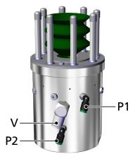
1. Connect the compressed air hose for releasing the positioning pin clamps to the compressed air connection (P1) using the plug connector.
