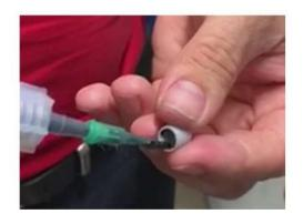
3. Use the tool to slide the cover cap onto the positioning pin. This ensures that there are no remaining air cushions between the positioning pin and the cover cap.
