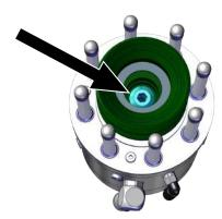
2. Screw on the new suction pad and sealing ring.
