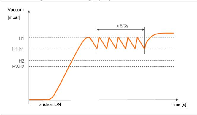
With the  $[\Box \Box \Box = \Box \neg]$  setting, continuous suction is deactivated, and the ejector continues in control mode despite a high leakage rate or control frequency greater than 6 times per 3 s.
