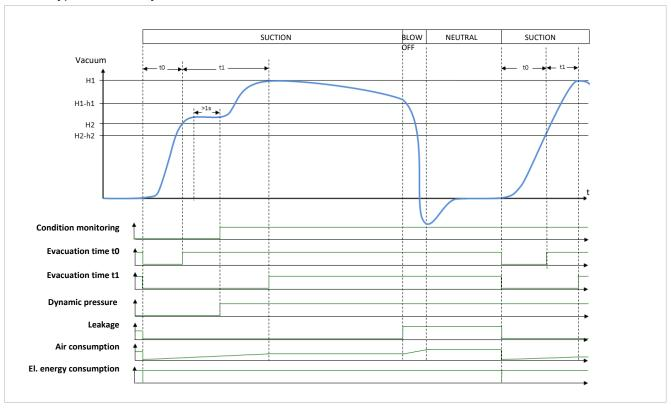
Handling cycle with leakage > L and readjustment:
