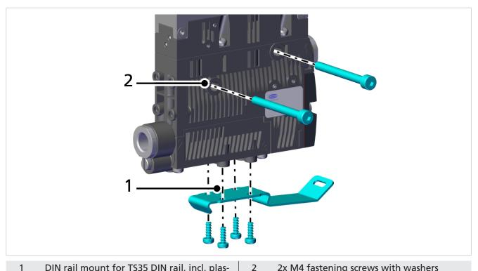
1 DIN rail mount for TS35 DIN rail, incl. plastic tapping screws Max. tightening torque 0.5 Nm
