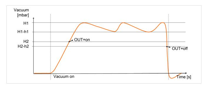
The ejector has an integrated air saving function and automatically regulates the vacuum in suction mode:
