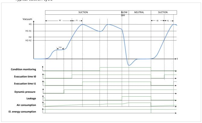
Handling cycle with very high leakage (H1 is not reached):
