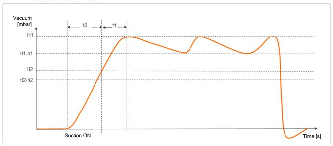
If the measured evacuation time t1 (from H2 to H1) exceeds the specified value [t-1], the "Evacuation time longer than t-1" condition monitoring warning is triggered and the system status light switches to yellow.
