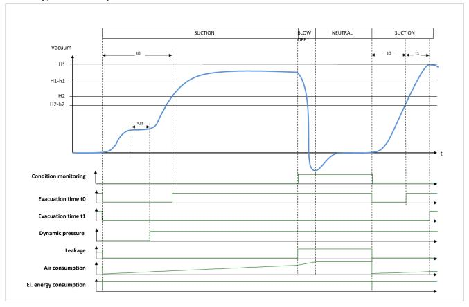
Handling cycle with excessive evacuation time t1:
