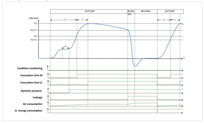
Handling cycle with dynamic pressure measurement and excessive leakage:
