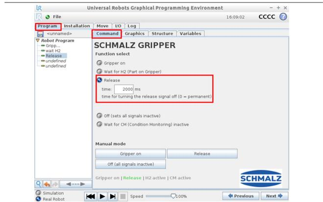
The gripper can be controlled manually via these buttons.
